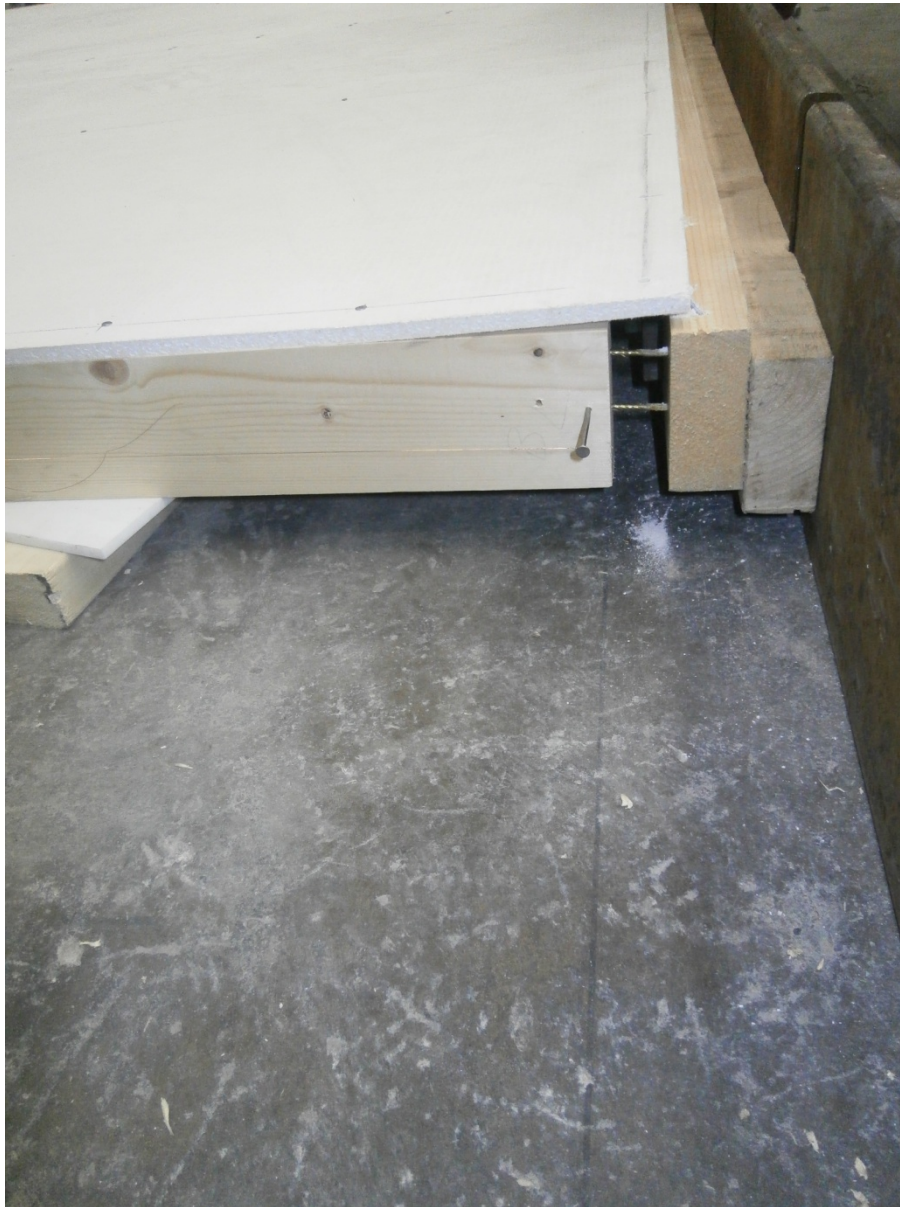
Plate 3 – Typical Mode of Failure after 0 kN Vertical Top Load Tests
