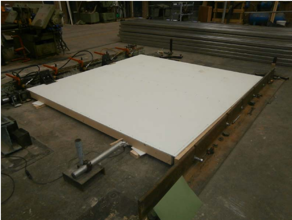
Plate 1 - General View of Racking Test Arrangement
