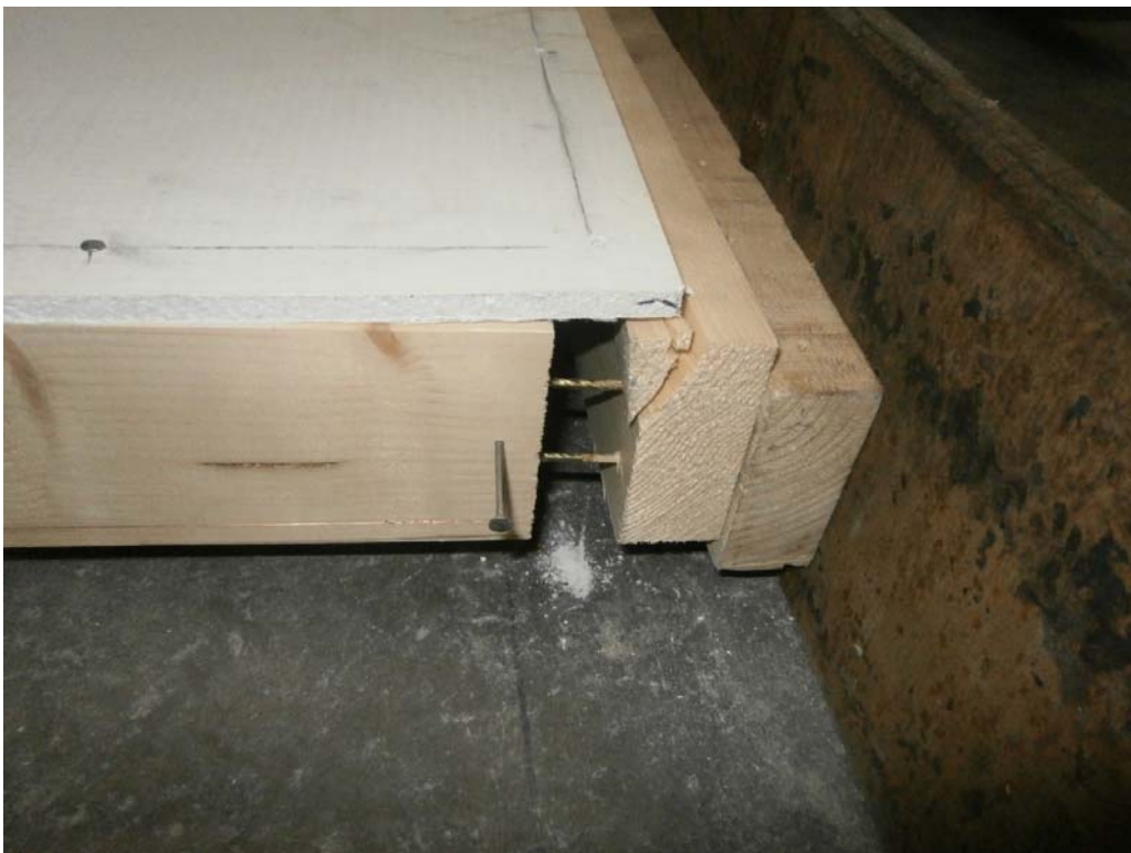
Plate 2 – Typical Mode of Failure after 0 kN Vertical Top Load Tests
