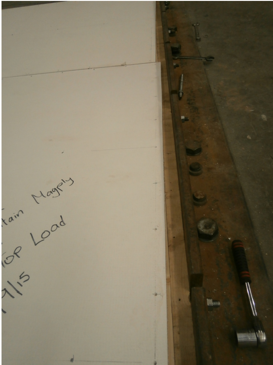
Plate 5 – Typical Mode of Failure after 5 kN Vertical Top Load Tests
