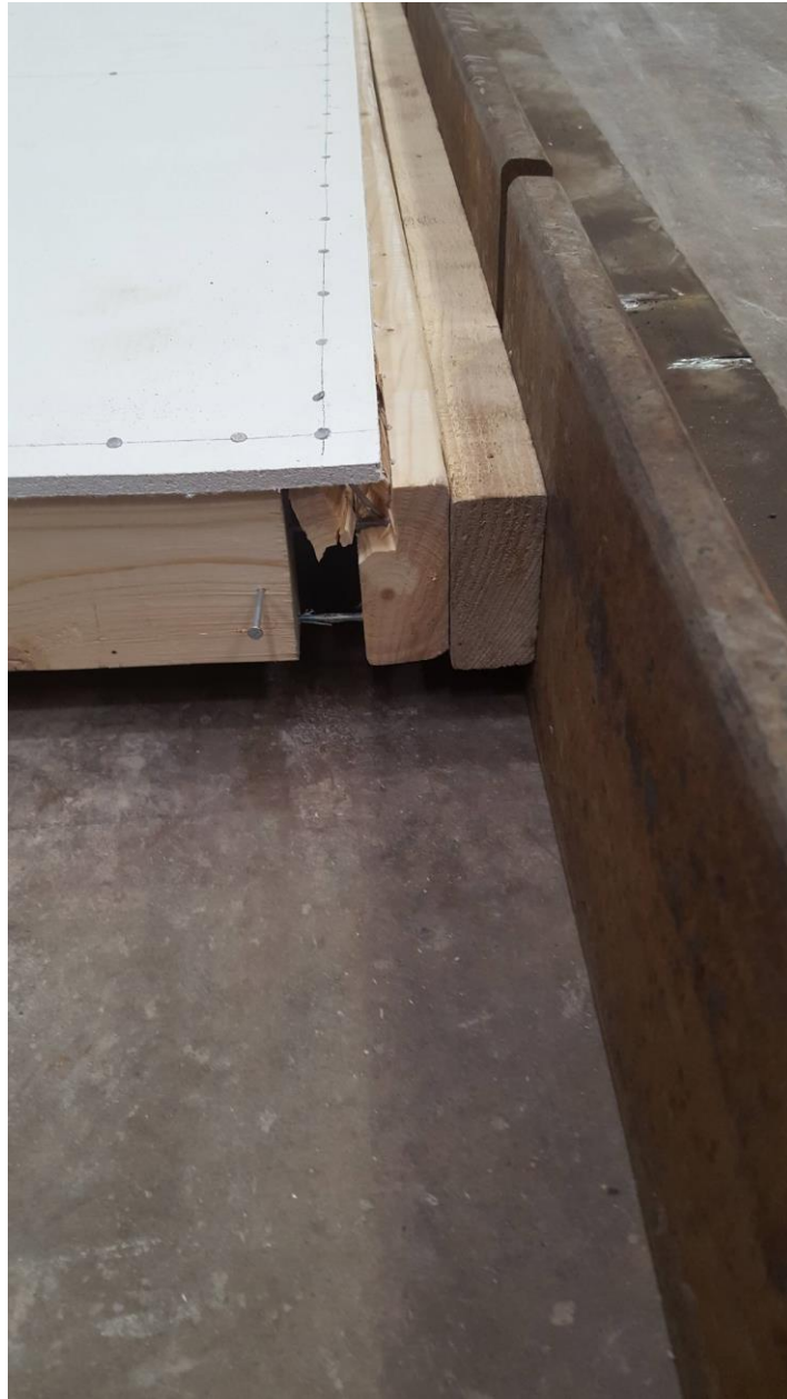
Plate 2 – Typical Mode of Failure after 0 kN Vertical Top Load Tests
